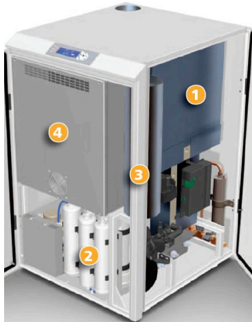
Figure 4: BlueGen Module incorporating an Solid Oxide Fuel Cell (1), water treatment system (2), gas cleaning system (3) and power management system [including grid connected inverter] (4) (CFCL 2009)
